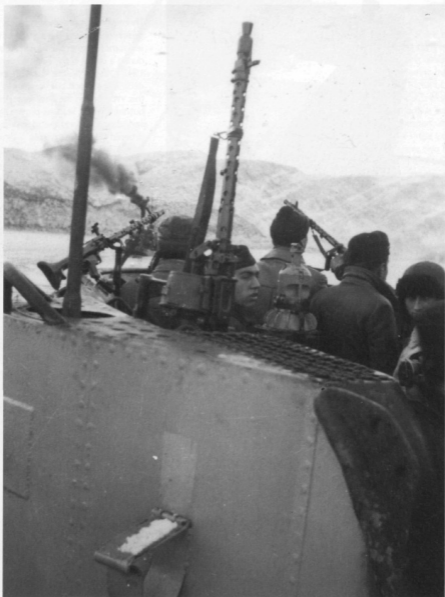
An interesting photograph showing the bridge of an unidentified U-boat. The bridge is heavily defended by three MG34 machine guns. The MG34 could be utilised in both a light and heavy role and had an effective range of 2000m (2188yds) and an impressive rate of fire of 800-900 rounds per minute. This weapon could undoubtedly deliver a formidable volume of fire and was particularly effective at combating low level aircraft attacks against U-boats.
